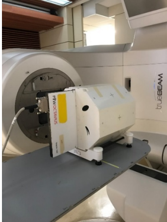
Figure 5. 10. PTW Octavius phantom utilized to compare the treatment planning dose verses the measured dose was set up on the treatment couch as shown.
